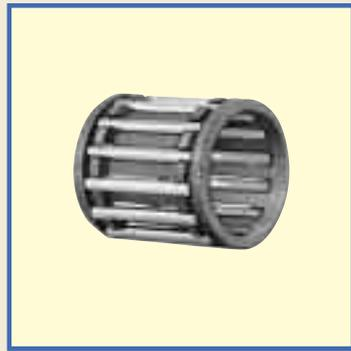
Needle Roller Cages for Engine Connecting Rods are used for motor cycles, small motor vehicles, outboard marines, snow mobiles, general-purpose engines, high-speed compressors, etc. that are operated under extremely severe and complex operating conditions such as heavy shock loads, high speeds, high temperatures, and stringent lubrication. Needle Roller Cages for Engine Connecting Rods are lightweight and have high load ratings and high rigidity as well as superior wear resistance.
