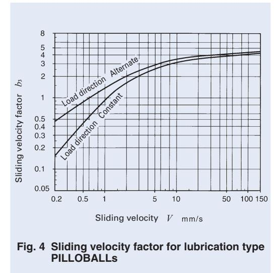
**Fig. 4 Sliding velocity factor for lubrication type PILLOBALLS**
