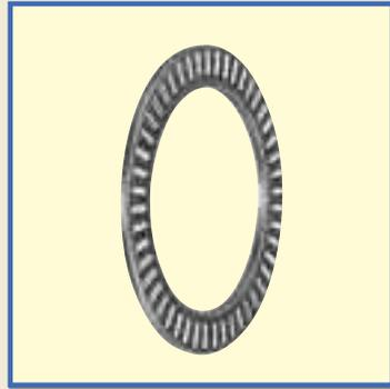
Thrust Bearings consist of a precisely made cage and rollers, and can receive axial loads. They have high rigidity and high load capacities and can be used in small spaces. Thrust Needle Roller Bearings use needle rollers, while Thrust Roller Bearings use cylindrical rollers.
