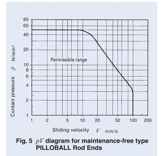
**Fig. 5  $pV$  diagram for maintenance-free type PILLOBALL Rod Ends**
