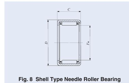
**Fig. 8 Shell Type Needle Roller Bearing**
