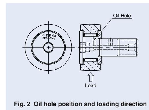
Fig. 2 Oil hole position and loading direction
