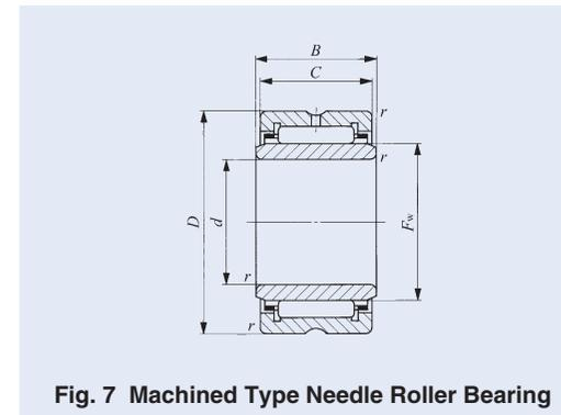
**Fig. 7 Machined Type Needle Roller Bearing**
