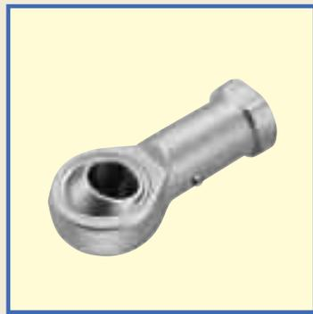
PILLOBALLS are compact self-aligning spherical plain bushings which can support a large radial load and a bi-directional axial load at the same time. PILLOBALL Rod Ends have either a female thread in the body or a male thread on the body, so they can be easily assembled onto machines. PILLOBALLS are used in control and link mechanisms in machine tools, textile machines, packaging machines, etc.
