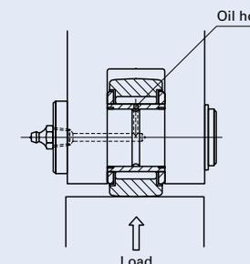
**Fig. 2 Position of oil hole and load direction**
