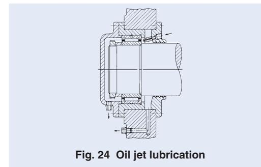
Fig. 24 Oil jet lubrication
