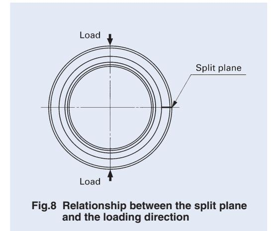
Fig.8 Relationship between the split plane and the loading direction
