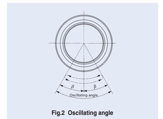
**Fig.2 Oscillating angle**
