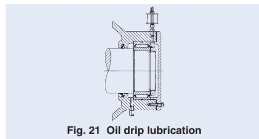
Fig. 21 Oil drip lubrication
