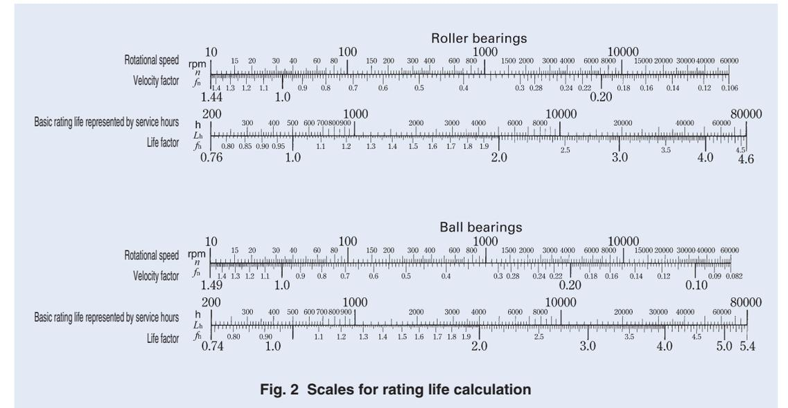
Fig. 2 Scales for rating life calculation
