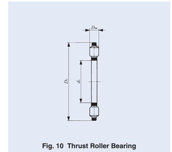
**Fig. 10 Thrust Roller Bearing**
