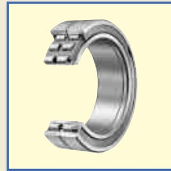
Roller Bearings, in which rollers are incorporated in double rows, are non-separable heavy-duty bearings. They can withstand not only radial loads but axial loads as well, which are supported at the contacts between the shoulders of inner and outer rings and the end faces of rollers. Therefore, they are most suitable for use at the fixing side of a shaft.
