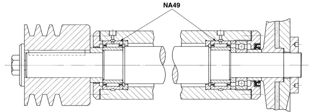
● Main spindle of drilling machine
