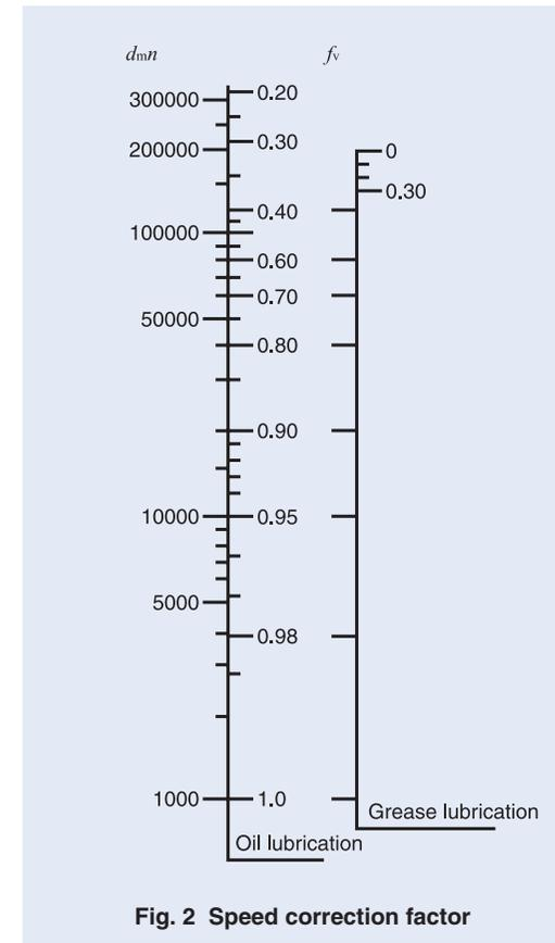
Fig. 2 Speed correction factor
