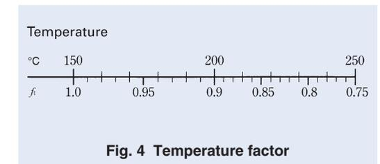
Fig. 4 Temperature factor
