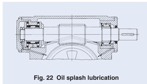
Fig. 22 Oil splash lubrication
