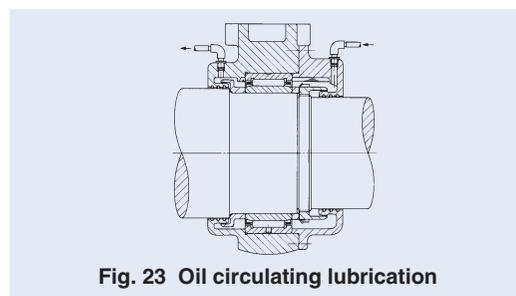
Fig. 23 Oil circulating lubrication
