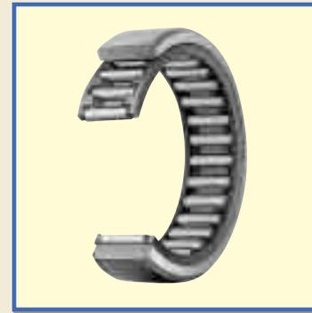
In Needle Roller Bearings with Separable Cage, the inner ring, outer ring and Needle Roller Cage are combined, and they can be separated easily. This type has a simple structure with high accuracy. In addition, the radial clearance can be freely selected by choosing an assembly combination. These bearings have excellent rotational performance, because Needle Roller Cages are used.
