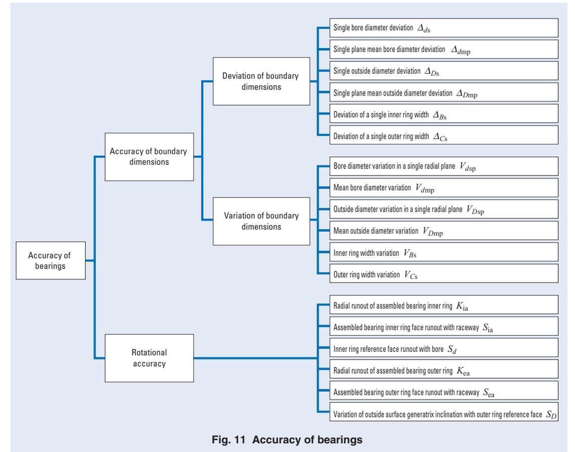
Fig. 11 Accuracy of bearings
