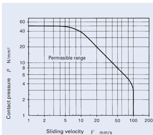
**Fig. 2  $pV$  diagram of lubrication type PILLOBALLS**
