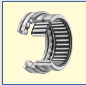
Combined Type Needle Roller Bearings are combinations of a radial bearing and a thrust bearing. Caged Needle Roller Bearings are used as radial bearings and Thrust Ball Bearings or Thrust Roller Bearings are used as thrust bearings. They can be subjected to radial loads and axial loads simultaneously.
