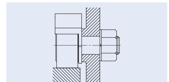
Fig. 7 Mounting of C-Lube Unit
