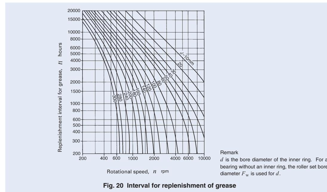
**Fig. 20 Interval for replenishment of grease**
