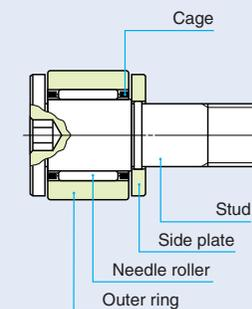
Note<sup>(1)</sup> In case of the stud diameter ( $d_1$ ) 5 to 10mm, a lubrication fitting is provided in the stud head hex hole. The stud diameter ( $d_1$ ) 12 to 30mm, a grease nipple is provided in the stud head hex hole.
