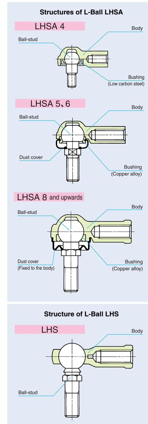
base grease, they have excellent lubrication and anti-dust properties and can run for long periods of time without re-lubrication.
